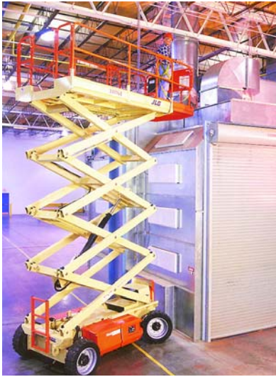
3369 LE is pictured above. 4069 LE is similar model with an additional scissor stack allowing a platform height of 40'.
